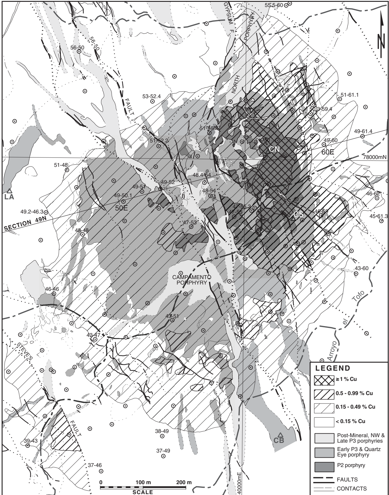
FIG. 13. Distribution of Cu grade at the surface, Bajo de la Alumbraera, before supergene leaching and enrichment, interpreted from near-surface drill hole assays and surface mapping of sulfides, limonite, and Cu oxides. Au distribution closely reflects Cu distribution, with Au (ppm)/Cu (%) varying from ~0.8 to ~1.6. Drill holes also shown, with numbers for selected holes referred to in text or other figures. CN = Colorado Norte, CS = Colorado Sur, LA = Los Amarillos, CB = Cerro Blanco.
