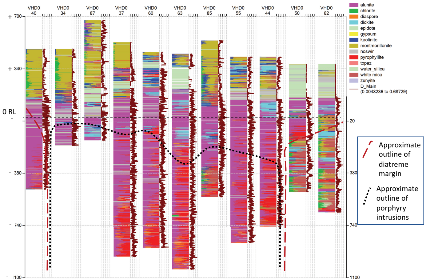
Fig. 8. Drill holes along SE-NW longitudinal section (as in Fig. 4b) arranged in pseudo-section showing relative spectral contribution from short wave infrared (SWIR) spectroscopy of samples at 1-m intervals with on-site ASD instruments. Plotted in aiSIRIS™ software provided by AusSpec. The approximate margins of the diatreme breccia and the porphyry intrusions are shown for reference.
