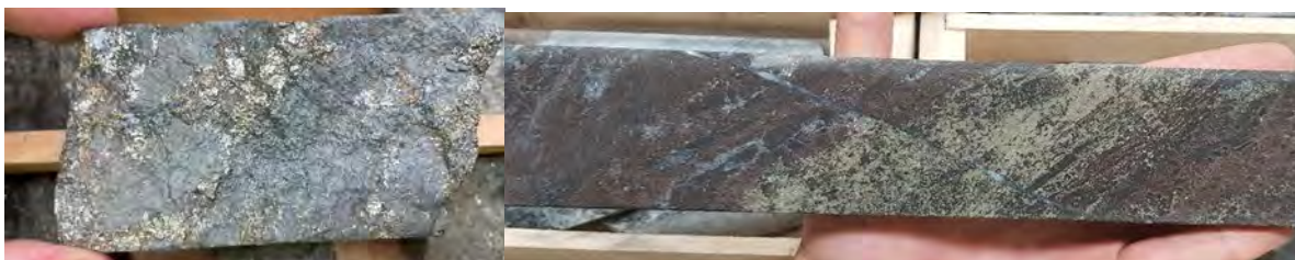
Fig. 6 [Left]: Ultrafine-grained, high-grade Au arsenopyrite that has behaved in a brittle manner, with fractures infilled with chalcopyrite and pyrite, Boliden ore. BOL-24 core.
