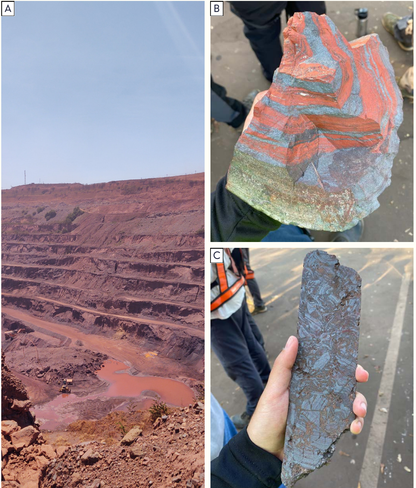
Figure 3: A - One of several pits at the Serra Norte deposit. B - Sample of jaspelites. C - Core sample of iron ore extracted from the deposit.
