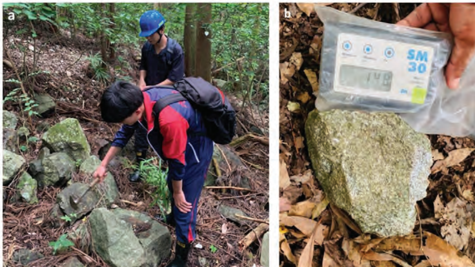
Figure 12 (a-b) Kawara skarn province outcrop and measurement of magnetic susceptibility of the skarn deposit related granodiorite intrusion.
