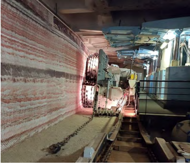
Figure 20 : Haveuse (Mining cutter) in surface
