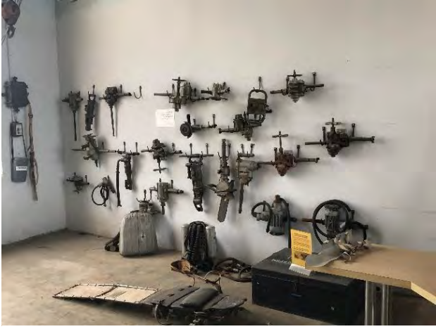
Figure 18 : Different types of Jackhammer
