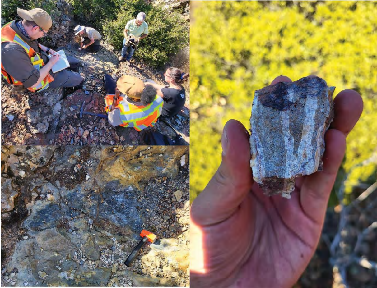
Figure 13: (Upper left) Outcrop containing massive sulfides and Ag-Au-Te sulfosalts that are part of the HS mineralization. (Lower left) Close-up of the sulfosalt-rich HS mineralization. (Right) Au-bearing amethyst vein (IS) crosscutting the HS hydrothermal event represented by vuggy quartz.
