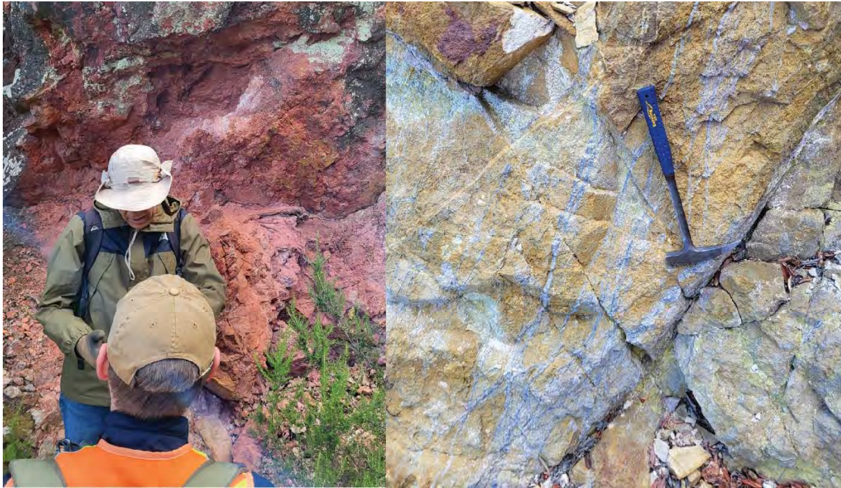
Figure 11: (Left) Advanced argillic alteration containing quartz and diaspore. (Right) Porphyry-style quartz stockwork crosscut by pyrite-bearing B-veins in the sericitic altered hornblende-biotite intrusion at Konos Hill.
