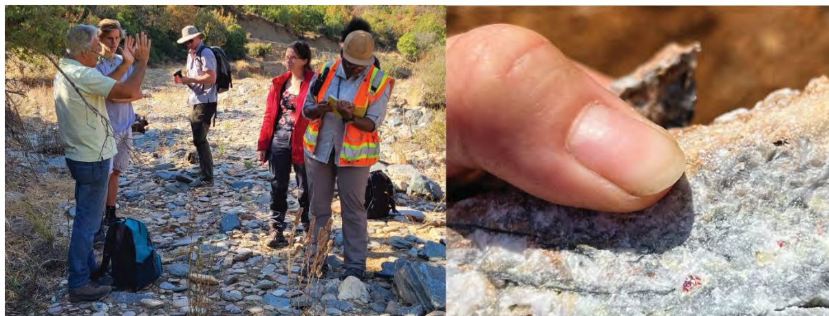
Figure 17: (Left) Participants discussing in the creek the origin of the mineralization formation. (Right) Close-up of the stibnite mineralization with the occurrence of realgar (red).
