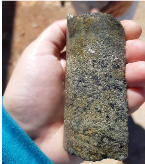
Figure 1: 25th May (Drill-core description) - South body target with ore minerals (pyrite, chalcopyrite and chalcocite)
