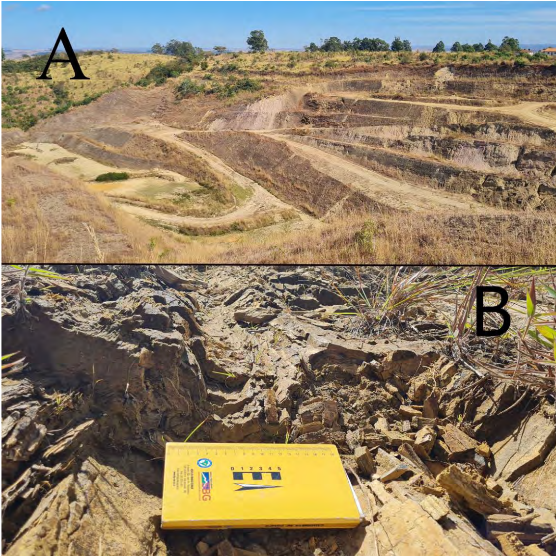
Figure 8: A – Photo of the open pit mine; B - apatite rich levels with approximately 5 cm of thickness (dark brown) and barren metasilites.
