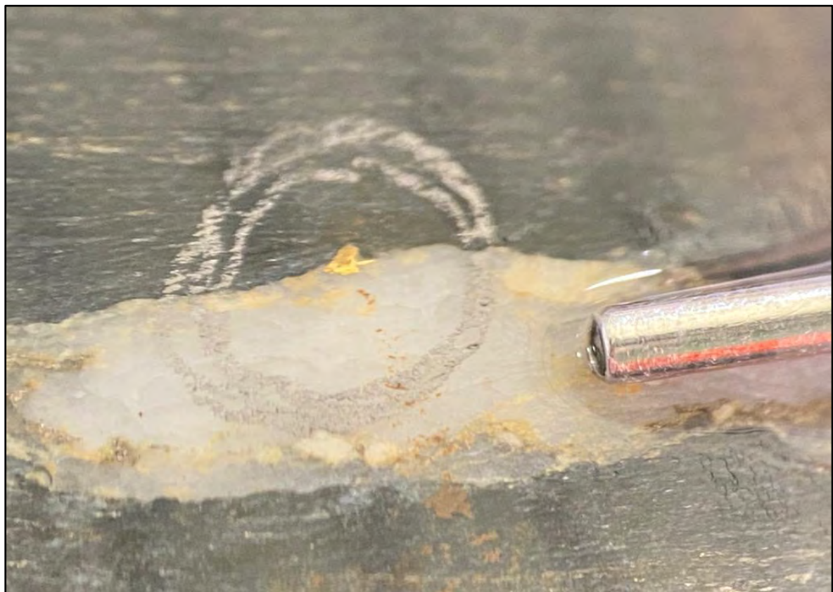
Figure 15: Gold grain associated to quartz boudin found on a drill core sample – Mina Morro do Ouro, Paracatu.
