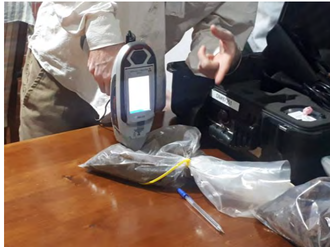
Figure 3 - Geochemistry analysis using an X-ray portable diffractometer
